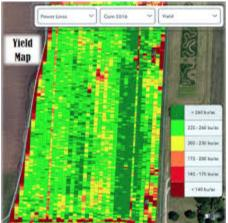
yield MAPS — These are generated by the GPS and other programs present in the harvesting equipment. The data collected will indicate ranges of bushels harvested per acre of a crop, telling you where the high levels and low levels of productivity are located, indicating where improvements can be made: different crop variety, increases in fertilization rates, confirming drainage issues or areas of compaction.
